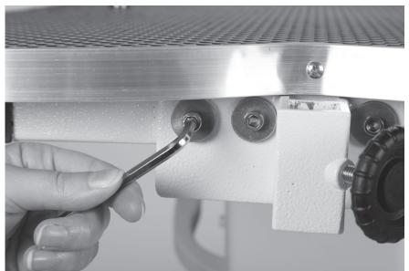
1. Connect the Grooming Arm Holder (A) to Table by lining up the holes on the Holder with the holes on the Table. Thread one Large Washer (C) and one Small Washer (D) onto each Screw (E). Tighten Screws to table.
